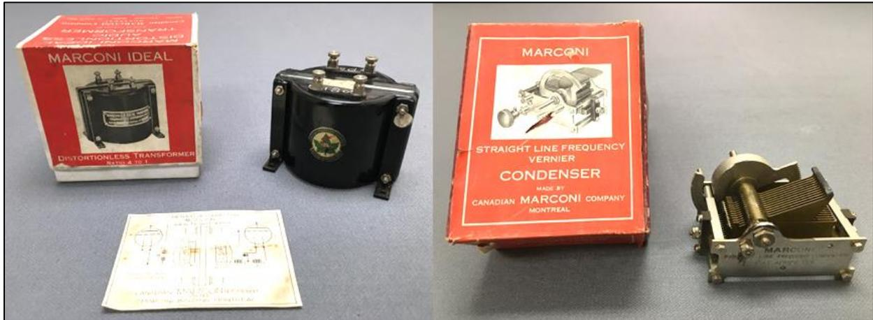
**Distortionless Transformer and Straight Line Frequency Condenser,
