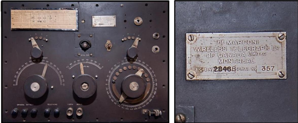
**Type 2846B Maritime Receiver; originally designed as a crystal receiver in 1918 and 1920; later converted to vacuum tubes (ca.1925). It may have kept its crystal detector as a back-up mode**
