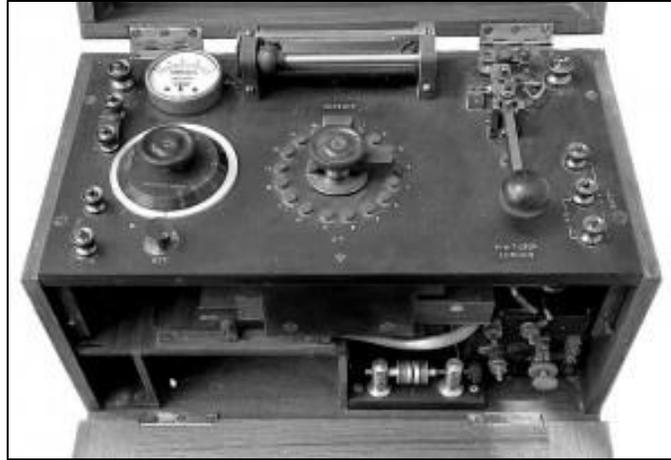
**Wireless Telegraphy (W/T) Trench Set 50 Watt D.C. (also known as the BF set). The spark gap is clearly seen at the bottom**
