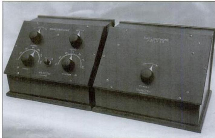
**Marconiphone Model 1 (Mk I) with its two-valve audio amplifier**
