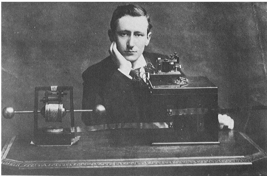
Marconi, 22, as he appeared in London in the spring of 1896. The Morse code sounder and two pieces of copper wire acting as the receiving antenna are on top of the black box on the right containing the coherer while, on the left, is the Hertzian dipole oscillator.
