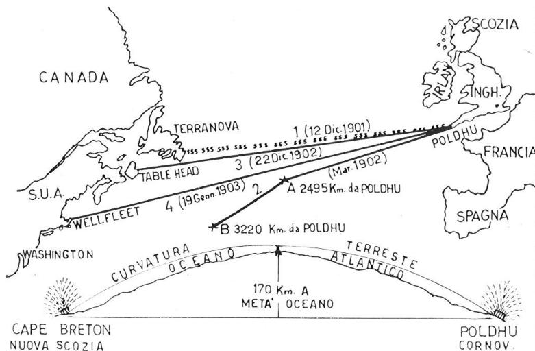
A sketch illustrating in Italian the main long distance experiments performed by Marconi in the early years of the last century. Points A and B correspond to the positions of a ship on which receiving apparatus were mounted. The lower part of the sketch shows the apparent line-of-sight problem faced by the early experimenters.
