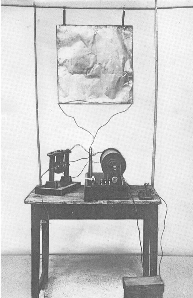
The first device developed by Marconi in Bologna in 1895 for wireless transmission. The antenna is a tin plate from an oil barrel. Another metal plate was laid on or buried in the ground. At the transmitting station, a spark gap (instrument on the table on the left) was connected between the two plates while at the receiving station the detector (a coherer, instrument on the table at the right) was connected between the plates.
